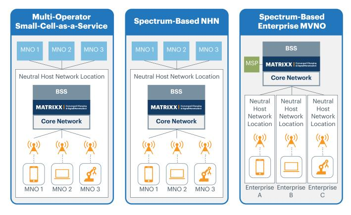
**Multi-Operator Small-Cell-as-a-Service** — In the first scenario, the NHN deploys services via small cells but using the frequency bands of upstream mobile network operators. There may be an opportunity to increase the upsell from the NHN by providing seamless, integrated Wi-Fi coverage in particular locations as well, monetization of this model is mostly driven by the MNO plans in place.
